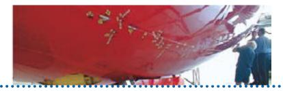
Lightning can also damage composite airplane structures if protection finish is not applied, properly designed, or adequate. This damage is often in the form of burnt paint, damaged fiber, and composite layer removal (see fig. 7).
