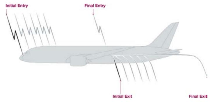
During the initial stages of a lightning strike on an airplane, a glow may be seen on the nose or wing tips caused by ionization of the air surrounding the leading edges or sharp points on the airplane's structure. This ionization is caused by an increase in the electromagnetic field density at those locations. In the next stage of the strike, a stepped leader may extend off the airplane from an ionized area seeking the large amount of lightning energy in a nearby cloud.
